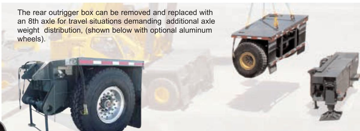
The rear outrigger box can be removed and replaced with an 8th axle for travel situations demanding additional axle weight distribution, (shown below with optional aluminum wheels).
