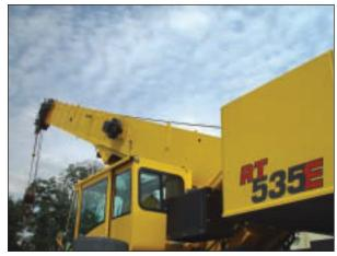
The RT535E incorporates a rectangular boom shape made from 100k.s.i. steel which eliminates weight and improves capacity compared to conventional shapes.
