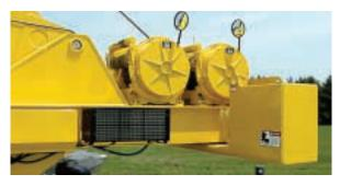
The RT600E uses a 11,250 lbs. pinned-on counterweight. Cable power is provided through Grove model HO30G-16G grooved drum hoists with 16,800 lbs. permissible line pull. Max line speed is 593 fpm. Both the main and optional auxiliary hoists have cable capacity up to 450 ft.
