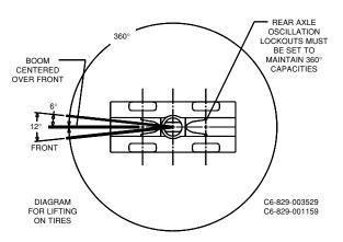
Bold lines determine the limiting position of any load for operation within working areas indicated.
