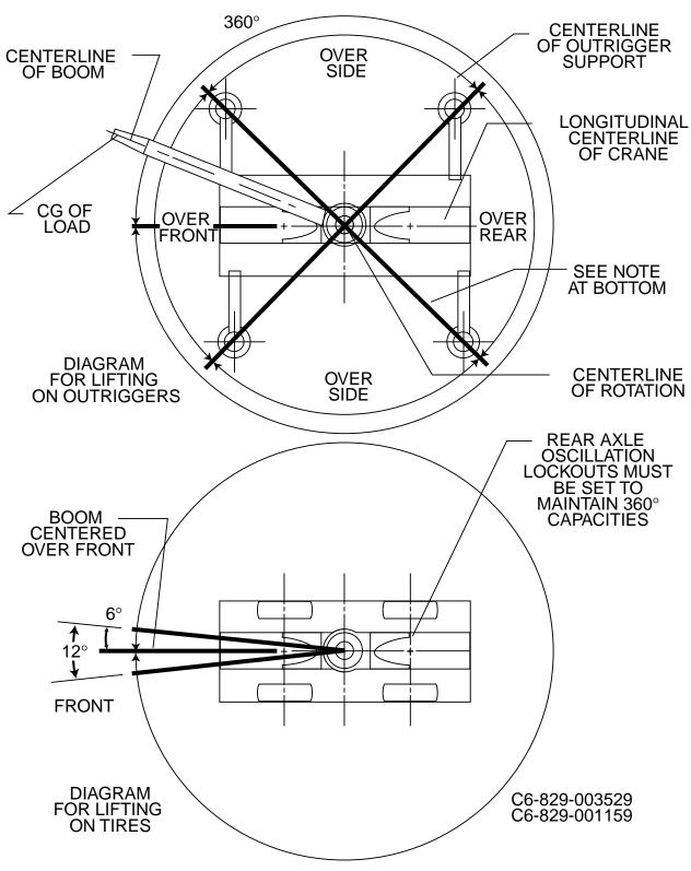
BOLD LINES DETERMINE THE LIMITING POSITION OF ANY LOAD FOR OPERATION WITHIN WORKING AREAS INDICATED
